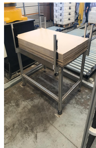
At each completed layer the robot picks up the intermediate layer carton from the warehouse (if required by the format)
