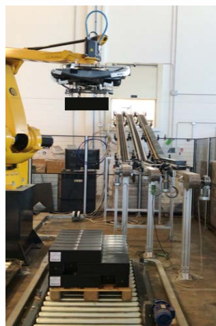
After picking up, the robot place the product on the relative pallet
